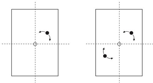
Pitch locations for 1 and 2 drop PRONTO systems are fully flexible and can be rotated about the injection point.
