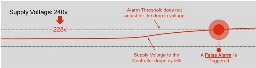
Altanium compensates for changes in voltage by adjusting alarm thresholds to avoid false alarms
