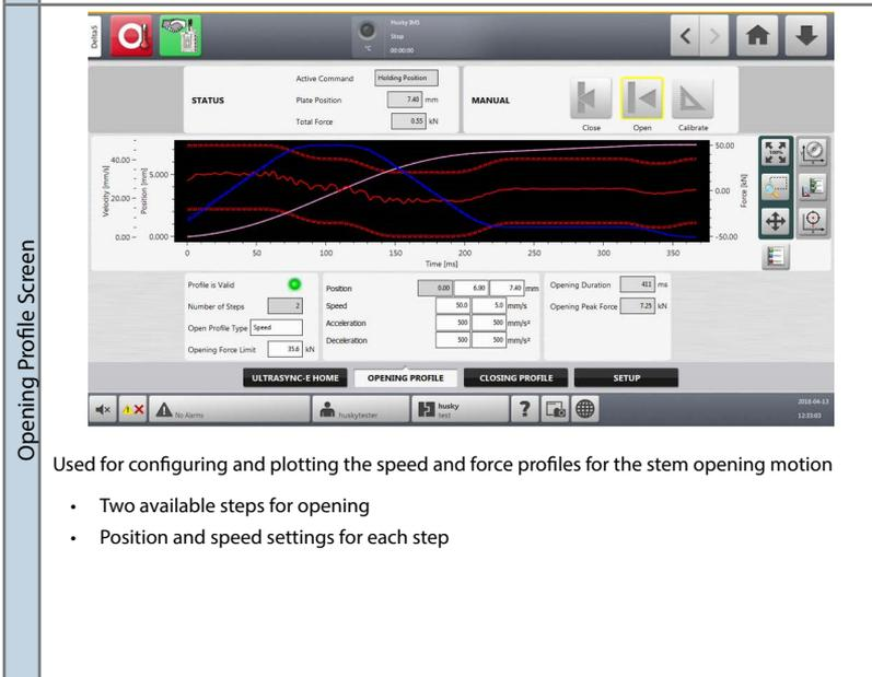
Used for configuring and plotting the speed and force profiles for the stem opening motion
