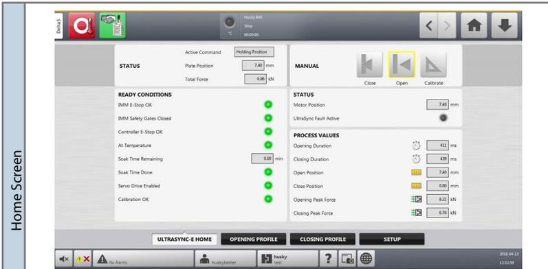
Displays indicators for all ready conditions and position, force and fault statuses as well as the manual controls for open and close and calibration
