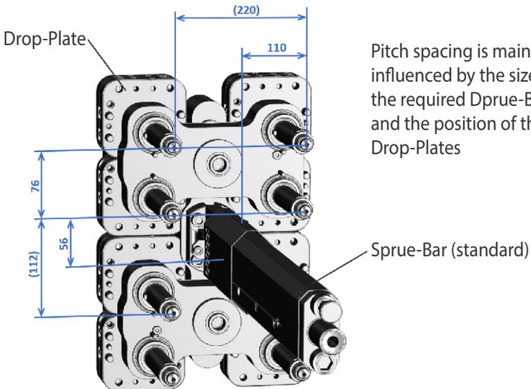
Pitch spacing is mainly influenced by the size of the required Dprue-Bar and the position of the Drop-Plates
