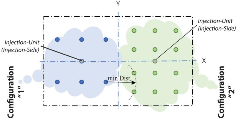
PRONTO-Multi Material (2K) consists of 2 separate manifolds. Any combination of the following listed layouts is possible. (Up-to 16+16 Drops)
