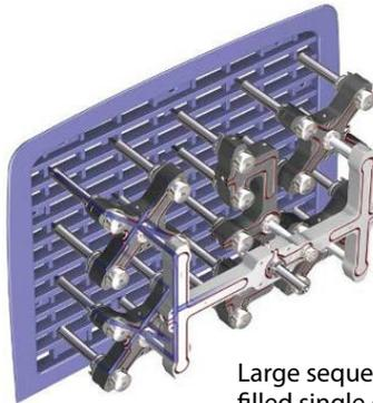
Large sequentially filled single cavity Automotive part
