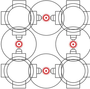
*Square configuration - to minimize core shifting in critical applications (If core shifting cannot be addressed with part / mold design)*
